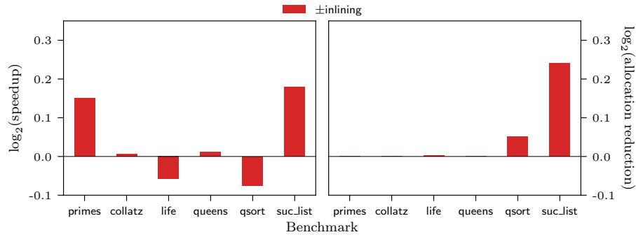
Fig. 4. Graphs showing the performance impact of our inliner when executed after PureCake’s demand analysis. Performance is clearly worse compared to Figure 3; therefore we do not pursue this approach.
