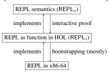
At the top is the semantic specification of the REPL. At the bottom is machine code implementing the REPL. In between is an implementation of the REPL as a function in logic. We describe the components of each layer in more detail below, then give an overview of the proof that each layer implements the one above it.
